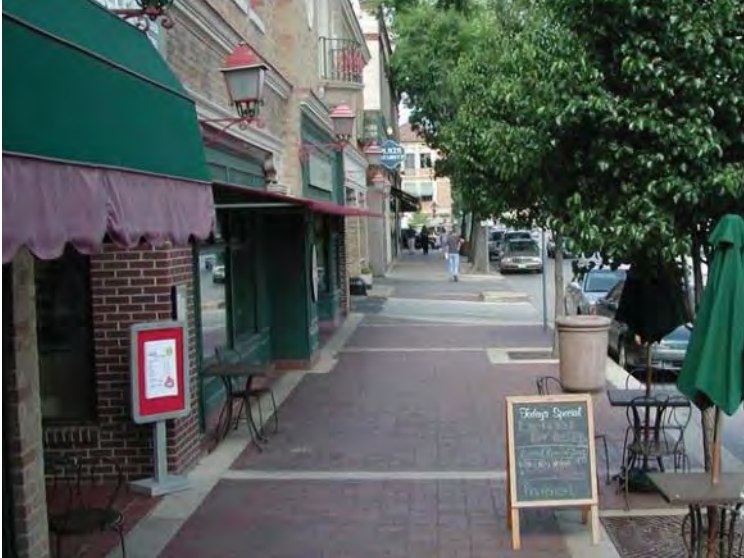
Driveway across sidewalk identified by material change
