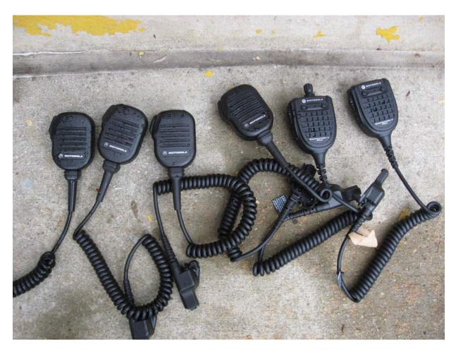
Motorola extended microphones used in testing model numbers NMN6193C, NMN6193BS03, NMN6191C, RMN5088A and RMN5066A
