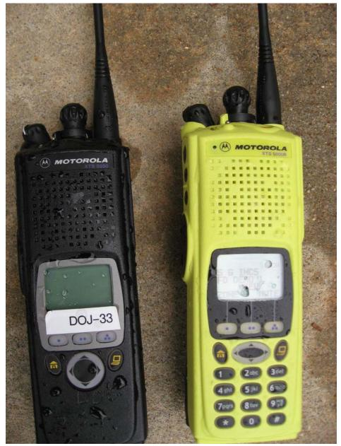
Radios used for field testing Motorola XTS 5000 Model II and XTS 5000R Model III with and without a variety of Motorola extension microphones
