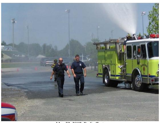
May 22, 2007, Radio Test Hydrant pressure through master stream fog nozzle – Heavy rain simulation
