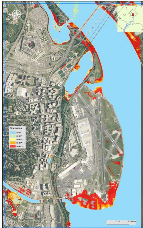
Figure 60: Projected Mean High-Water Scenario, Sea Level Rise for Ronald Reagan Washington National Airport, 2100 205
