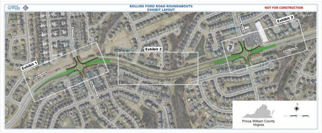
The Rollins Ford Road Roundabout Project involves the design and construction of two single-lane roundabouts at the intersections of Rollins Ford Road and Song Sparrow / Yellow Hammer Drive, and Rollins Ford Road and Estate Manor Drive. The proposed improvements would also reconfigure Rollins Ford Road between Song Sparrow / Yellow Hammer Drive and Estate Manor Drive from two lanes in each direction to one lane in each direction, with the existing outside lane removed through pavement striping.
